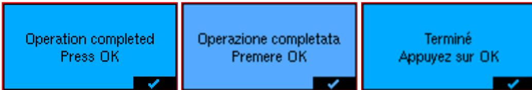
7. Turn off the vehicle, restore the pipes and restore the engine connections: once the cleaning operation is complete, the machine asks whether to proceed with emptying its hoses (strongly recommended) or to terminate the operation
