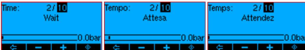
4. After setting the nebulization times, insert the sprayer into the **AIR** tank of the machine to start the **calibration/priming** procedure and press **ok**: the procedure pushes all the air out of the machine circuit, to stabilize the pressure of 4 bar that will be maintained throughout the treatment
