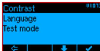
4. Set the desired contrast with the keys + / - and press **ok**: the suggested contrast is **20**
