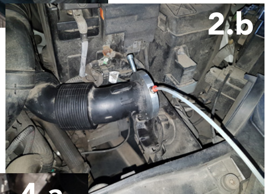
Spray head clamped on the air filter line inlet
